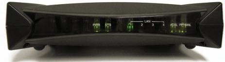
**NOTE:** You will have five lights visible on the front of the modem. Four will be solid green, and one “LAN” light will be flashing. If at any time the modem does not look as it should, please refer to the troubleshooting portion of this guide to further assist you.
