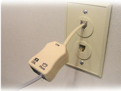
Plug devices (phone, fax, satellite dish, answering machine) into the filter in the “Phone” jack. Repeat on all the phone jacks that are in use in your home.
